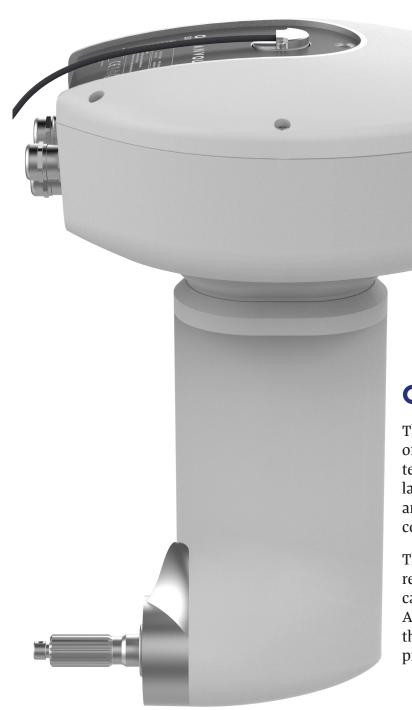
"The Oceanvolt SD system has a patented, flexible mounting to attach the motor to the sailboat hull to absorb vibrations."
