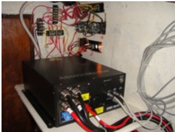
The Motor Compartment (clockwise) Batteries & Wire Platform, Battery Chargers, Motor Controller, and Motor
