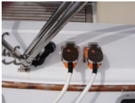
Shore Power Inlets - Two 30 Amp Lines
