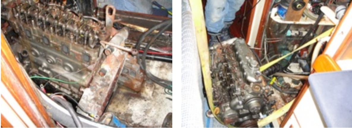
Engine Compartment - During Removal
